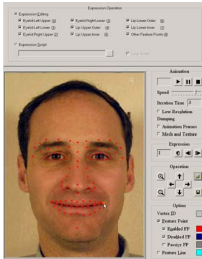
Fig. 12.18. The expression editing interface. The red dots are the feature points which a user can click on and drag. (From Zhang et al. [46], with permission.)
