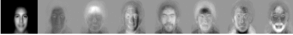
Fig. 7.2. Eigenfaces: the average face on the left, followed by seven top eigenfaces. From Turk and Pentland [36], with permission.
