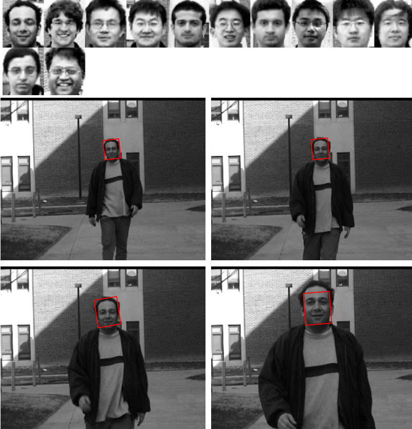
Fig. 8.2. Database-0. First row: the face gallery with image size of 30 \times 26 . Second and third rows: four frames in one probe video with image size of 320 \times 240 ; the actual face size ranged approximately from 30 \times 30 in the first frame to 50 \times 50 in the last frame. Note that the sequence is taken under a well controlled condition so there are no significant illumination or pose variations between the gallery and the probe.
